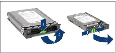
Figure 25: Unlocking the 3.5-inch and 2.5-inch HDD modules
